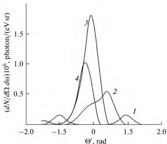
**Fig. 3.** Effect of increasing the angular density of the TR upon the emission of 200-keV electrons from a carbon target at different angles: (1) 90°; (2) 60°; (3) 30°; (4) 15°. The photon energy is 50 eV.
