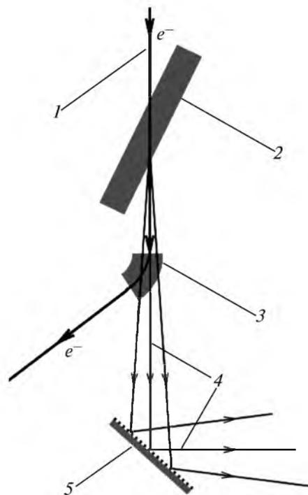
**Fig. 5.** Scheme of a possible source of VUR based on transition radiation at glancing interaction: (1) electron beam; (2) target; (3) magnet; (4) VUR; (5) diffraction grating.
