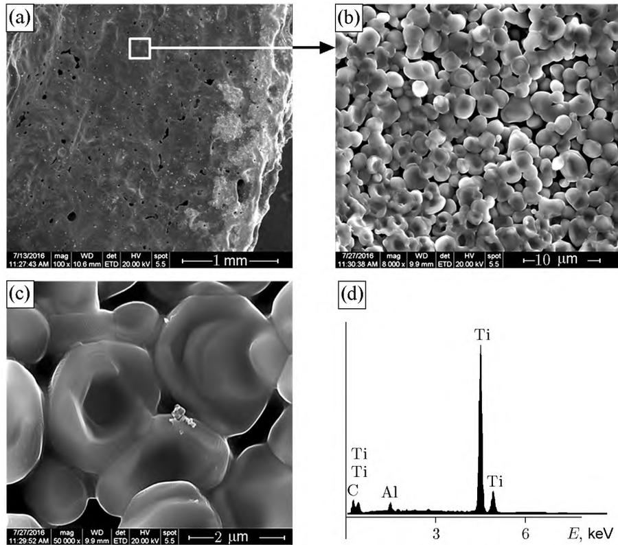
**Fig. 6.** Structure of the peripheral region (SHS process zones) of the Ti–Al–C sample after treatment with an electron beam: (b, c) morphological features of TiC crystals at different zooms; (d): 26.64% CK, 3.84% ALK, and 69.52% TiK.
