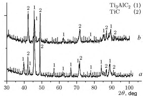
**Fig. 5.** Diffractograms of the SHS products: ignition of the mixture by electromagnetic radiation in an argon medium at a pressure of 5 atm (curve *a*) and ignition of the mixture by a high-power electron beam in vacuum (curve *b*).
