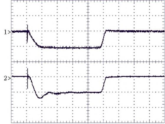
**Fig. 2.** Current oscillograms of the “SOLO” device [10]: (1) discharge current  $I_d$ ; (2) electron beam current  $I_g$ ; the abscissa axis is 50  $\mu\text{s}/\text{div}$ , and the ordinate axis is relative units per division.
