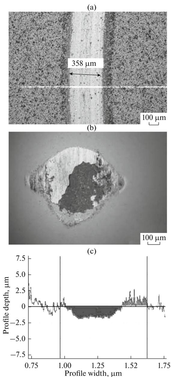
**Fig. 6.** Wear track on the (a) surface of coating and (b)  $\text{Al}_2\text{O}_3$  ball counterbody and (c) profile of the wear groove of the coating after testing of  $(\text{TiAlSiY})\text{N}$  coating (batch 1).
