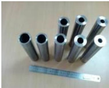
**Figure 1.** Tube billets for screw rolling.
