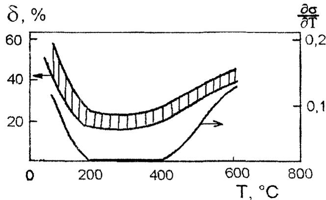
Fig. 3. The temperature dependence of the relative elongation of AISI304 and AISI316 steels irradiated up to fluence  $3 \cdot 10^{24}$  neutron/m<sup>2</sup> (dotted area) and  $\partial \sigma / \partial T$  that is the slope angle of flow stress temperature dependence in an unirradiated state.
