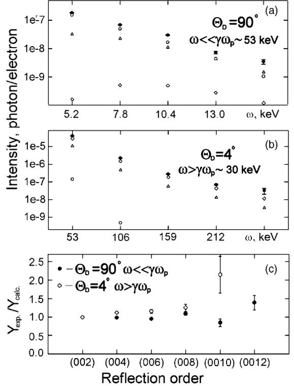
Fig. 3. Dependence of the radiation intensity on the photon energy: experimental spectrum ( $\bullet$ ) and calculation results of PXR ( $\Delta$ ), DB ( $\diamond$ ) and DTR ( $\circ$ ). (a)  $\Theta_D = 90^\circ$ ; (b)  $\Theta_D = 4^\circ$ ; (c) the ratio of the experimental and total (PXR + DB + DTR) calculated radiation yields.
