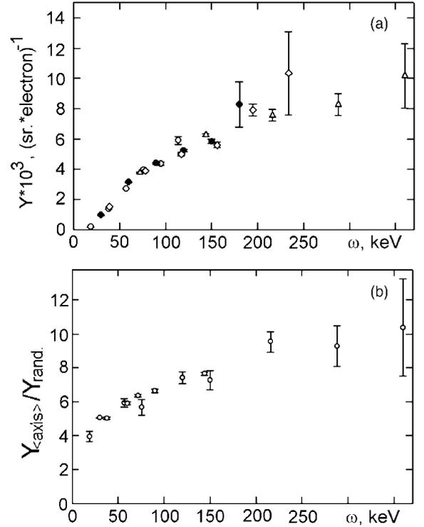
Fig. 5. (a) Spectrum of the angular density of the  $\langle 110 \rangle$  channeling radiation intensity for four detection angles: ○ –  $\Theta_D = 11.16^\circ$  and  $\omega_1 = 19$  keV; ● –  $\Theta_D = 7.18^\circ$  and  $\omega_1 = 30$  keV; ◇ –  $\Theta_D = 5.58^\circ$  and  $\omega_1 = 39$  keV; △ –  $\Theta_D = 2.94^\circ$  and  $\omega_1 = 72$  keV; (b) The ratio of the radiation yields for disoriented and oriented crystals.
