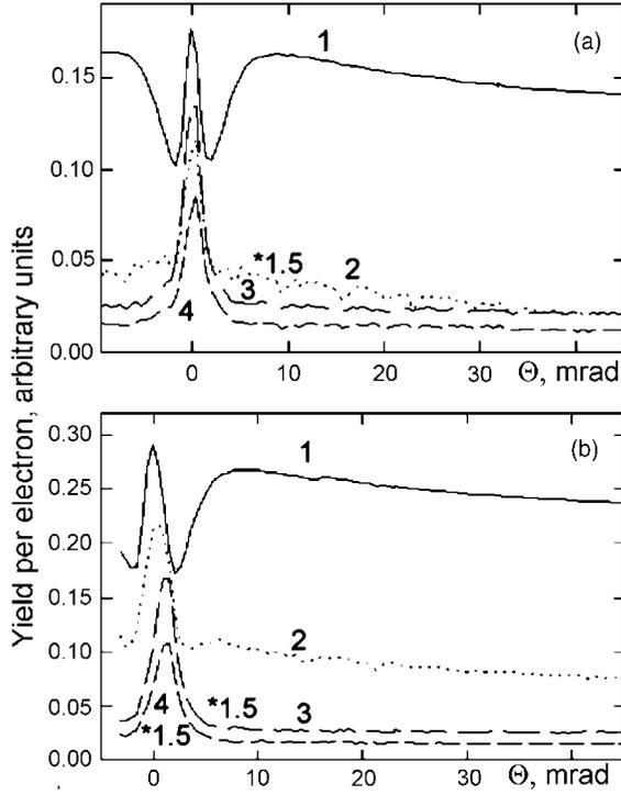
Fig. 4. Orientation dependences of the photon yield: silicon crystal with  $\langle 110 \rangle$  orientation;  $t = 0.52$  mm;  $E_0 = 500$  MeV. 1 – total radiation energy; 2 –  $\omega \geq 0.5$  MeV; 3 –  $\omega = 29$  keV; 4 –  $\omega = 36.5$  keV. (a)  $\alpha = 0$ ;  $\theta_o \sim 0$  mrad;  $\Delta\theta_o = \pm 0.1$  mrad;  $\theta_s = \pm 0.6$  mrad; (b)  $\alpha = 0$ ;  $\theta_o \sim 1.2$  mrad;  $\Delta\theta_o = \pm 0.1$  mrad;  $\theta_s = \pm 1.5$  mrad.
