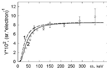
Fig. 6. Spectrum of the angular density of the radiation intensity for the disoriented crystal: ○ – experiment, the curves – calculation: 1 – without angular dependence of the bremsstrahlung suppression, 2 – angular dependence of the bremsstrahlung suppression is taken into account.
