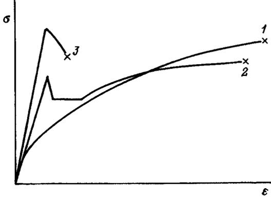
FIG. 1. Typical strain curves ( $\sigma$  — load,  $\varepsilon$  — deformation) for reactor steels at test temperatures below  $0.3T_m$  ( $T_m$  — melting temperature). 1 — Initial (unirradiated) material, 2 — material irradiated to “low” doses ( $10^{-2}$ – $10^{-1}$  dpa), 3 — material irradiated to doses above 1 dpa.
