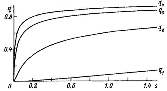
FIG. 2. Fraction of dislocations overcoming obstacles in the dynamic regime versus the initial dislocation velocity.  $q_1, q_2, q_3,$  and  $q_4$  correspond to the following values of the density of obstacles:  $p_1=10^{-4}\%$ ,  $p_2=10^{-3}\%$ ,  $p_3=10^{-2}\%$ , and  $p_4=10^{-1}\%$ , increasing as a result of irradiation.
