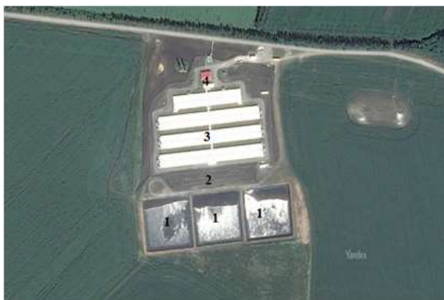
Fig. 1. A typical scheme of a pig-breeding complex on the territory of the Korochansky district of the Belgorod region. 1-Lagoons for the liquid fraction of manure, 2- Valliers for walking animals, 3-Rooms for keeping pigs, 4-Utility rooms
