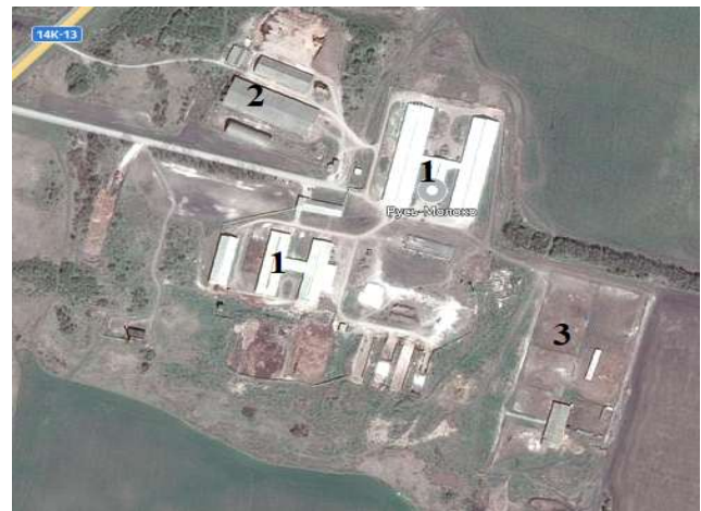
Fig. 2. Scheme of an agricultural enterprise for breeding large horned cattle on the territory of the Korochansky district Belgorod region. 1 - Premises for the maintenance of cattle, 2-Utility rooms, 3- Lagoons for the liquid fraction of manure
