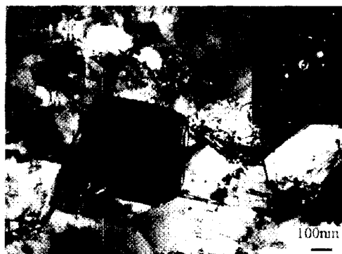
Figure 1. Microstructure of extruded MA754.
