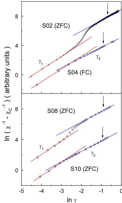
Fig. 5. The plots of  $\ln(\chi^{-1} - \chi_C^{-1})$  vs.  $\ln \tau$  for the samples S02–S10 in different cooling regimes, corresponding to the 3D percolation system with  $\gamma_1 \approx \gamma_p$  and the 3D Heisenberg system with  $\gamma \approx \gamma_H$ . The arrows mark the temperature  $T_1$ . The solid lines represent linear fits.
