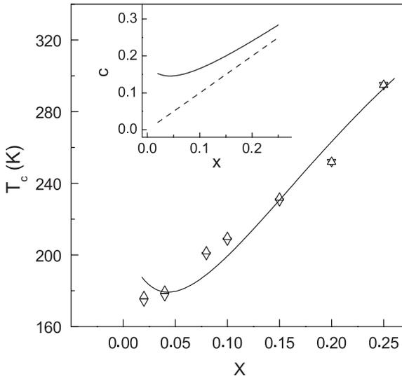
Fig. 2. Dependence of  $T_C$  on  $x$  for LBM0 determined from the inflection points of the interpolated curves of  $\chi_{ZFC}(T)$  and  $\chi_{FC}(T)$  ( $\nabla$  and  $\Delta$ , respectively). The solid line is evaluated with Eq. (2) as described in the text. Inset: Dependence of  $c$  on  $x$  calculated with Eq. (1) (the solid line). The dashed line represents the concentration of  $Ba^{2+}$ .
