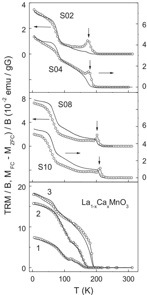
Fig. 3. Temperature dependence of  $\text{TRM}/B$  (solid lines) and  $(M_{\text{FC}} - M_{\text{ZFC}})/B$  (symbols) for the LBMO samples S02–S10 (upper and middle panels) and for LCMO (lower panel) with  $x = 0$  and  $c \approx 0.19$  (plots 1),  $x = 0.05$  and  $c \approx 0.15$  (plots 2) and  $x = 0.15$  and  $c \approx 0.20$  (plots 3) [4]. The arrows mark the average values of  $T_{\text{C}}$ , determined from  $\chi_{\text{ZFC}}(T)$  and  $\chi_{\text{FC}}(T)$ , in Fig. 2.
