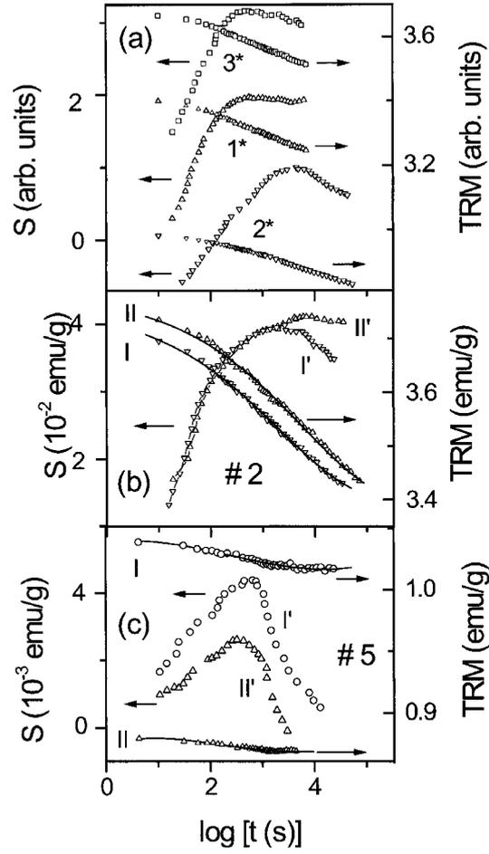
**Figure 6.** Dependences of TRM and  $S$  on  $\log t$  (a) for the samples 1\* at 80 K, 2\* at 65 K and 3\* at 75 K, measured after a wait time of  $t_w = 1.8 \times 10^3$ ,  $3.4 \times 10^3$  and  $3.5 \times 10^3$  s, respectively, (b) for sample 2 at 90 K after  $t_w = 3.6 \times 10^3$  s (I, I') and  $1.1 \times 10^4$  s (II, II') and (c) for sample 5 at 200 K (I, I') and 240 K (II, II') after  $t_w \approx 10^3$  s.
