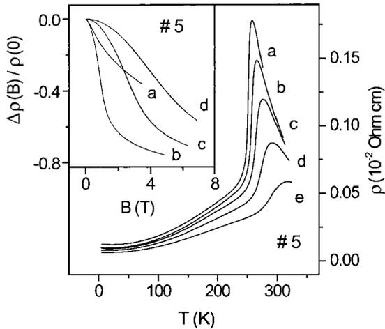
**Figure 4.** Dependence of the resistivity on temperature observed in sample 5 ( $x = 0.3$ ) for  $B = 0$  (line a), 1 T (line b), 2 T (line c), 4 T (line d) and 8 T (line e). Inset: dependence of the relative magnetoresistance on the magnetic field for  $T = 244$  K (line a), 258 K (line b), 273 K (line c) and 290 K (line d).
