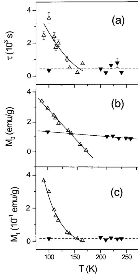
**Figure 8.** Temperature dependences of  $\tau$  (a),  $M_0$  (b) and  $M_1$  (c) for LCMO with  $x = 0.05$  (sample 2, open symbols) and 0.30 (sample 5, closed symbols). The solid lines are guides for the eye.
