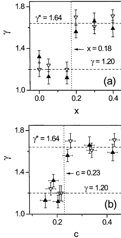
**Figure 3.** The critical exponent  $\gamma$  plotted for different  $x$  (a) and for corresponding values of  $c$  (b). The closed symbols represent the data obtained for the A samples [23] and the open symbols for the B samples (this work).
