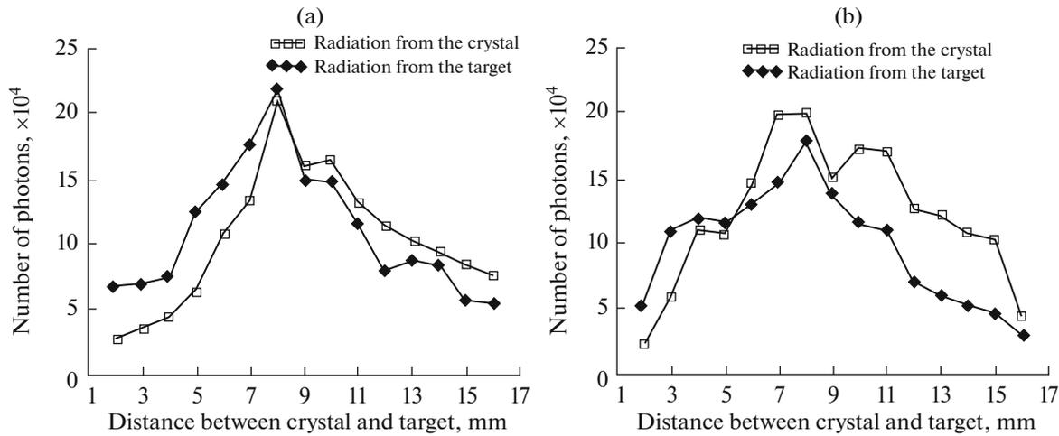
**Fig. 4.** Dependence of the yield of characteristic X-ray radiation upon heating and cooling of the crystal on the distance between the crystal and the target. (a, b) Demonstrate the results of measurements in two symmetrical positions of the X-ray detector.
