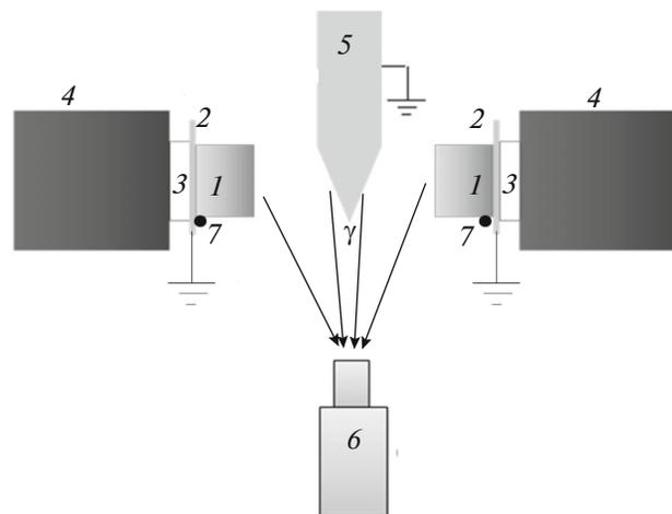
**Fig. 5.** Schematic diagram of the experimental setup: (1) pyroelectric crystals, (2) grounded conductive pad, (3) Peltier element, (4) heater, (5) target, (6) X-ray detector, and (7) digital thermometer.
