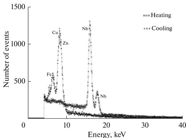
**Fig. 2.** X-ray spectra measured upon heating and cooling of the pyroelectric crystal; the distance between the crystal and the target is 8 mm.
