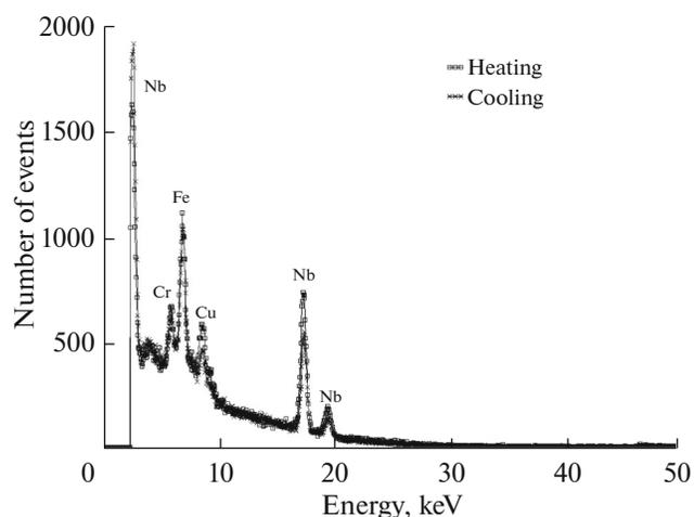
**Fig. 6.** X-ray spectra of the two-crystal source with a conical brass target, measured upon heating and cooling of the crystals.
