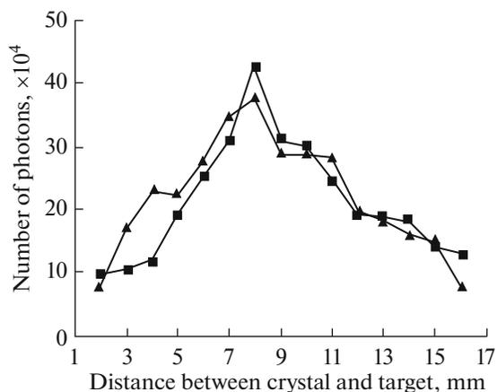
**Fig. 3.** Dependence of the total number of photons recorded by the spectrometer for one heating–cooling cycle on the distance between the crystal and the target. The measurements were carried out for two symmetrical positions of the X-ray detector.
