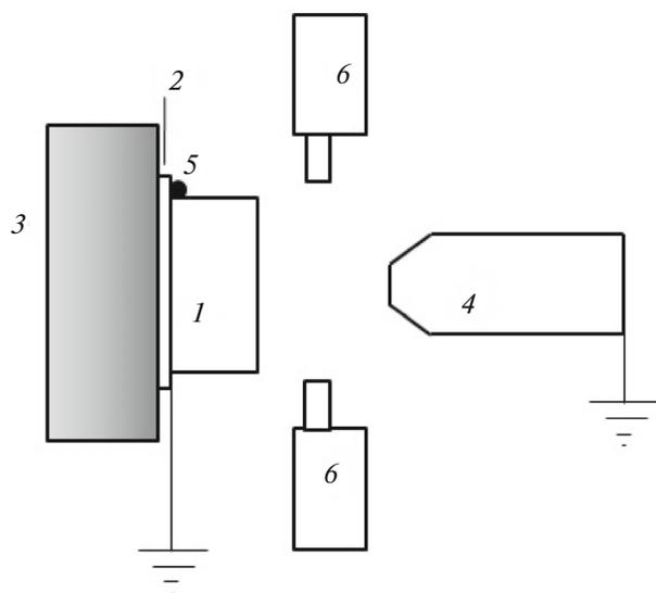
**Fig. 1.** Schematic diagram of the experiment with a single-crystal source: (1) pyroelectric crystal, (2) Peltier element, (3) cooler, (4) target, (5) digital thermometer, and (6) X-ray detector.
