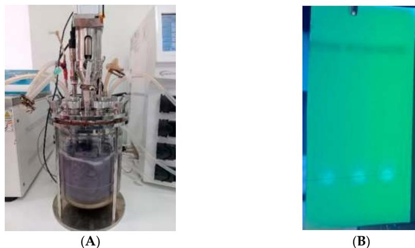
**Figure 6.** Illustration of cultivation of *J. lividum* strain VKM B-3705D by batch submerged method in Biocanvas LFD V1.5L bioreactor, Centrion, Republic of Korea (A) and the result of qualitative analysis by thin-layer chromatography (TLC) (B).
