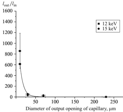
**Fig. 3.** Focusing power of capillaries versus the diameter of the output opening for different electron energies (the solid line depicts an exponential fit to the obtained data).
