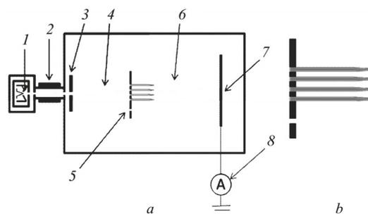
**Fig. 1.** Diagram of experiment (a) and holder with glass capillaries (b): 1) electron gun; 2) system of electromagnetic lenses; 3) collimator; 4) electron beam; 5) movable holder with goniometer; 6) electron beam transmitted through the capillary; 7) copper screen coated with scintillator powder; 8) Keithley 6482 picoammeter.
