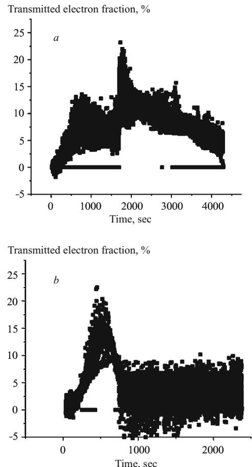
**Fig. 2.** Time dependence of the 12 keV electron current passing through capillaries Nos. 1 (a) and 3 (b), whose parameters are given in Table 1.
