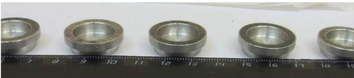
**Fig. 4** Photograph of the tear test specimens
